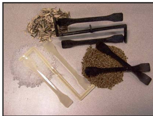
Biomass (upper left) compounded with resin (lower left) produces c2renew's biocomposite material (lower right) which can be molded into parts for end use companies
